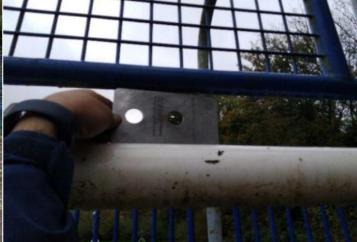
**Finding:** The item fails to meet the requirements of BS EN 15312 4.4.2.1 head and neck entrapment in the framework
