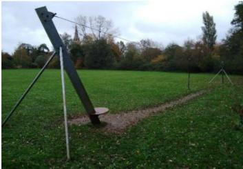
Finding: The height of the seat is less than 350mm when loaded and does not meet the requirements of BS EN 1176 ground level when loaded with 69.5kg Part 4
